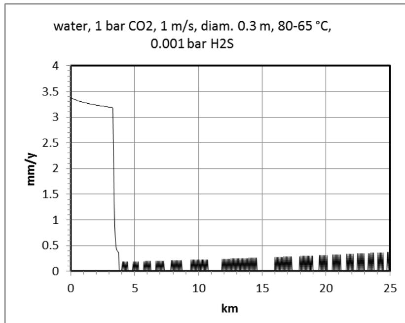
Fig. 9. Effect of a linear temperature profile, temperature gradient 0.6 °C/km, showing loss of stability of the  $\text{FeCO}_3$  layer in the presence of 0.001 bar  $\text{H}_2\text{S}$ .
