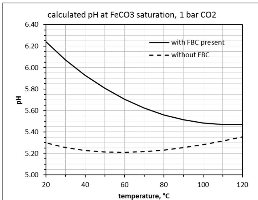
Fig.4. pH at  $\text{FeCO}_3$  saturation as function of temperature.
