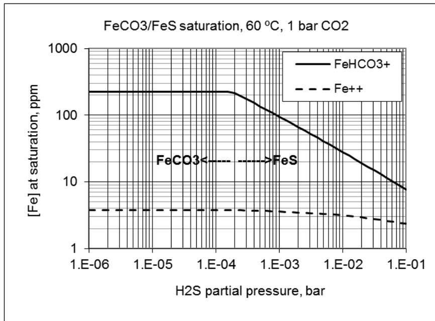
Fig. 8. Example of change from carbonate to sulphide precipitation by changing H<sub>2</sub>S partial pressure, at constant CO<sub>2</sub> pressure of 1 bar, at 60 °C.
