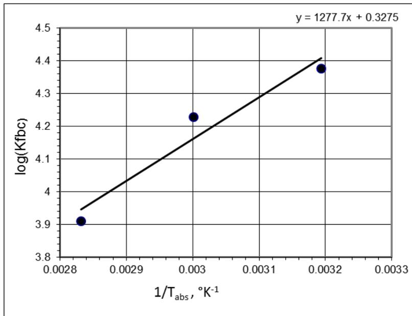
Fig.1. Arrhenius plot of  $K_{FBC}$  derived from Dugstad's experiments.
