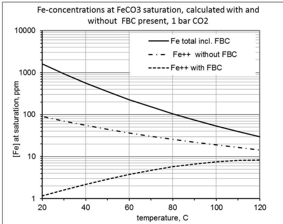
Fig. 2 . Total dissolved Fe concentrations at FeCO<sub>3</sub> saturation at 1 bar CO<sub>2</sub> as function of temperature, calculated with and without taking FBC into account.
