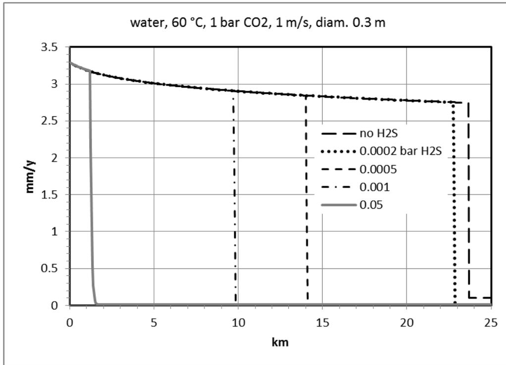
Fig. 7. Example of effect of H<sub>2</sub>S partial pressure on the location where scale can be formed. Water, 60 °C, pipe diameter 0.3 m, 1 bar CO<sub>2</sub>, 1 m/s.
