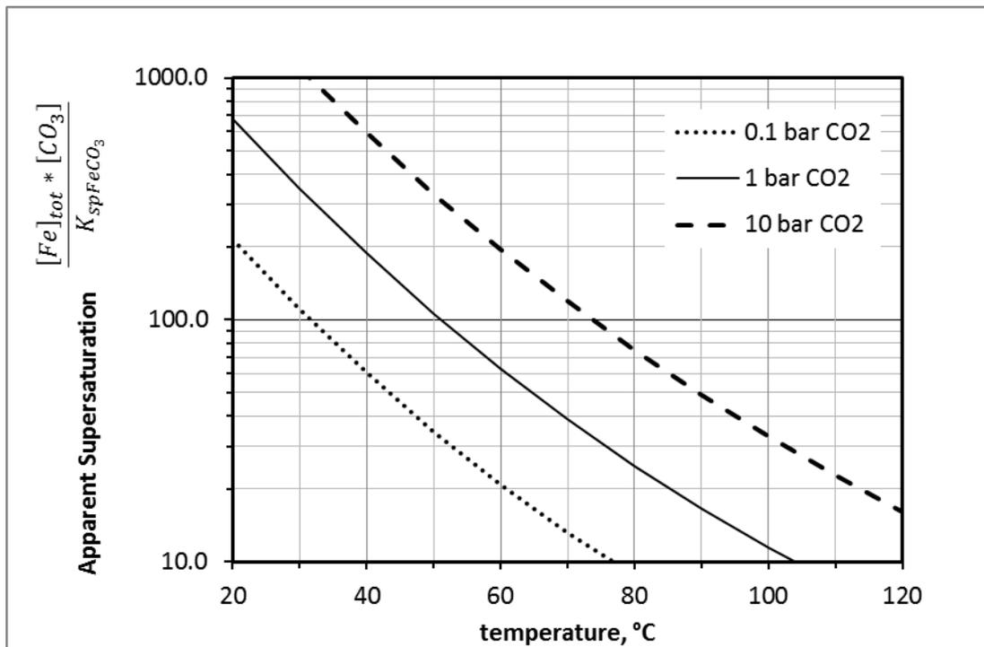
Fig. 3. Apparent supersaturation as function of temperature, calculated by taking the total dissolved Fe as being  $\text{Fe}^{2+}$ , at 1 bar  $\text{CO}_2$ .
