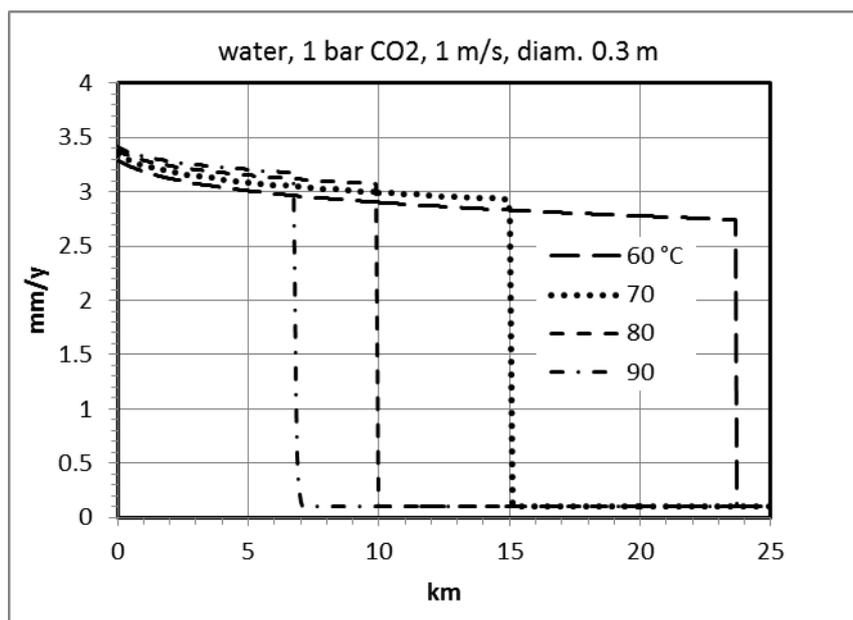
Fig. 5. Example of effect of temperature on formation of protective  $\text{FeCO}_3$  layer.
