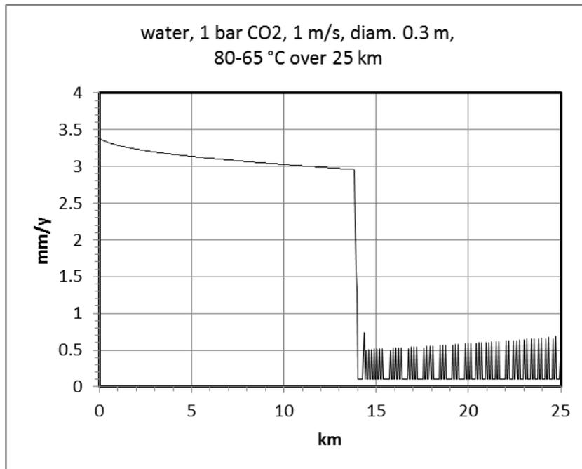
Fig. 6. Effect of a linear temperature profile,  $0.6\text{ }^{\circ}\text{C}/\text{km}$ , showing loss of stability of the  $\text{FeCO}_3$  layer.
